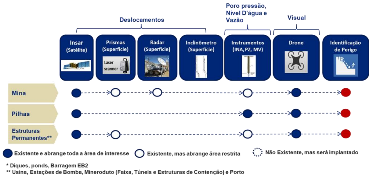
Figure 10: Schematic image of monitoring tools per structure and flow for hazard identification.
