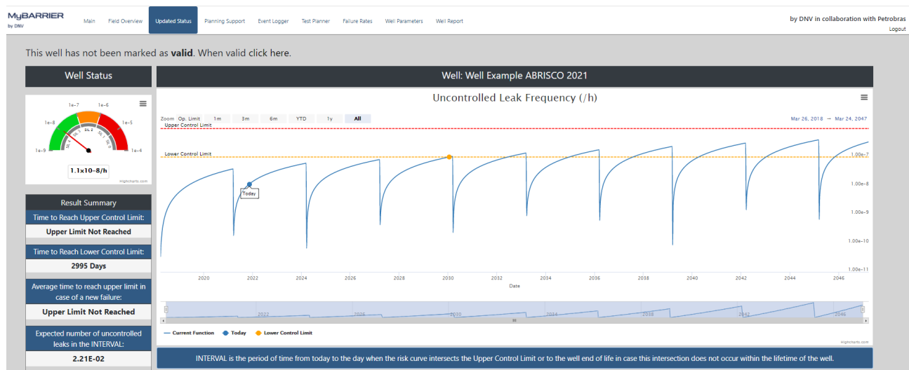
Figure 2 - Frequency of Uncontrolled Leak for Example Well without any Detected Failure
