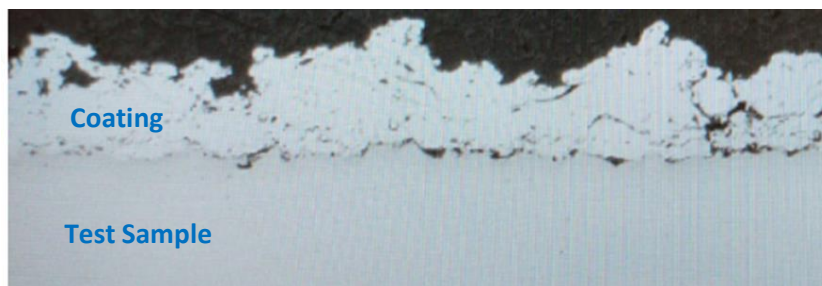
Fig. 6 – Microstructure of the coating
