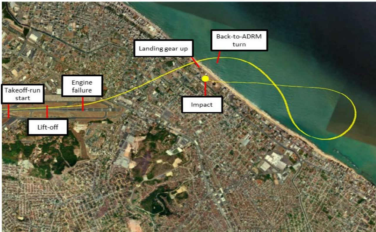
Figure 7 – Flight trajectory according to the flight data recorder [25].
