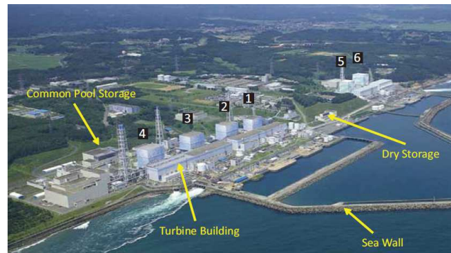
Figure 2 – Fukushima Daiichi building diagrams [4]
