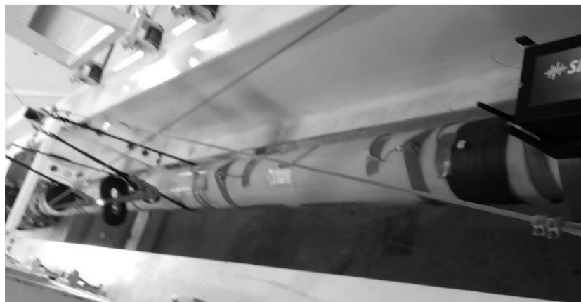
Figure 4 – 4" riser – tension-tension test rig
